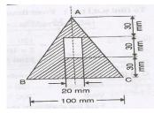
Q.10 Find the M.I. of a hollow section shown in figure about an axis passing through its c.g. or parallel to x-x axis.
